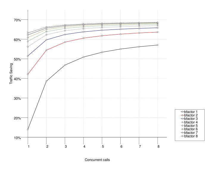
The results show a saving of 15.79% with only one concurrent call and with batching disabled (bfactor 1), that quickly improves with more concurrent calls (due to trunking).
